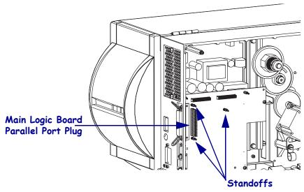
**9.** With the PSII device, take the cable and PSII board, go to the electronics side of the printer and plug the parallel port socket of the PSII board into the parallel port plug on the main logic board.
