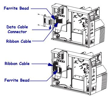
• For the *PAX* series, access the electronics by removing the mounting screws from the printer's PCB access panel and sliding the panel out.
