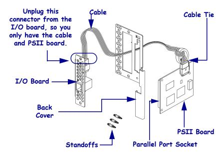
**8.** As shown in this illustration, insert the short ends of each standoff into the holes on the main logic board until you hear a click.
