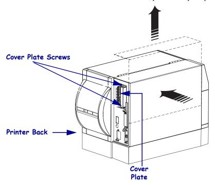
**6.** On the back of the printer, use the flat blade screwdriver to remove the screws and the cover plate.
